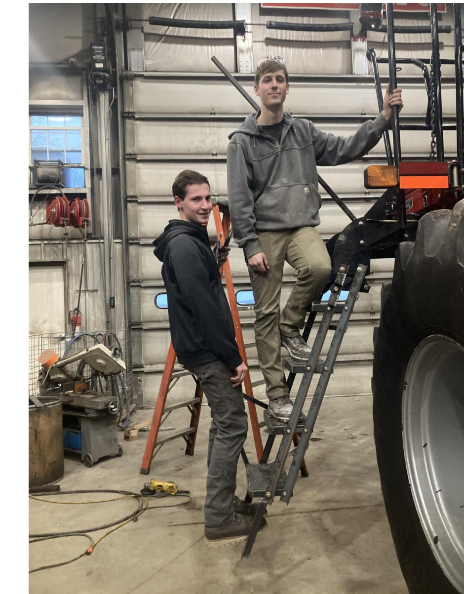
Two group members testing the prototype's weight capacity.
